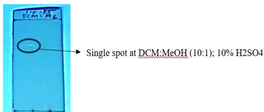
Figure 2. Separation of the EtOAc fraction of Aptos sp. and its bio-profile spot.
