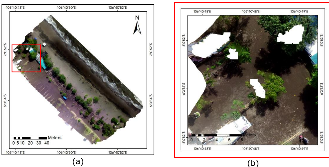
Figure 4. Orthophoto map of the coastal area of Cinta Beach, Tangerang Regency (a) and snapshot of the perforated section on the orthophoto (b).
