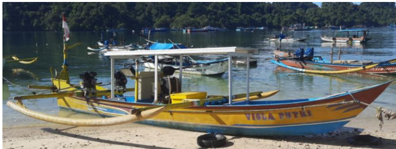
Figure 3. Small fishing vessel with solar powered chiller on board.
