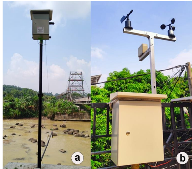
Figure 4. (a) Water level device (AWLR); (b) automatic weather station (AWS) which was tested at the laboratory.
