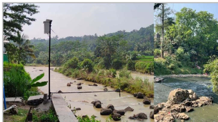
Figure 5. Several instruments are employed to continuously measure the flow of water in streams at observation locations located upstream of the Cikeas - Cileungsi watersheds. The measurement system is equipped with at least one water level sensor (Ultrasonic) and data.
