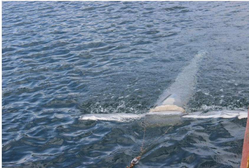
Figure 2. Manta net with a 15 x 25 cm 2 opening and a 200 µm mesh (original photo).
